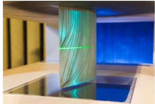
Photograph of airfoil equipped with pressure probes. Impact of laser sheet can also be seen
